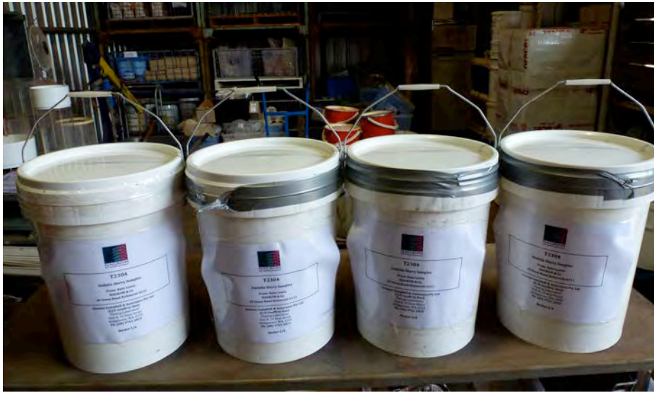
PLATE 1: 20 L drums containing tailings samples 'as-received' at GCA Testing Laboratory (Bridgetown) as supplied by Nagrom (Kewdale)
