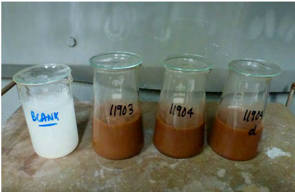
PLATE 6: Net-Acid-Generation (NAG) testing on pulps (-75 \mu\text{m} ) using 15 % \text{H}_2\text{O}_2 (@ pH 4.5). First boiling step shown following ageing overnight.
