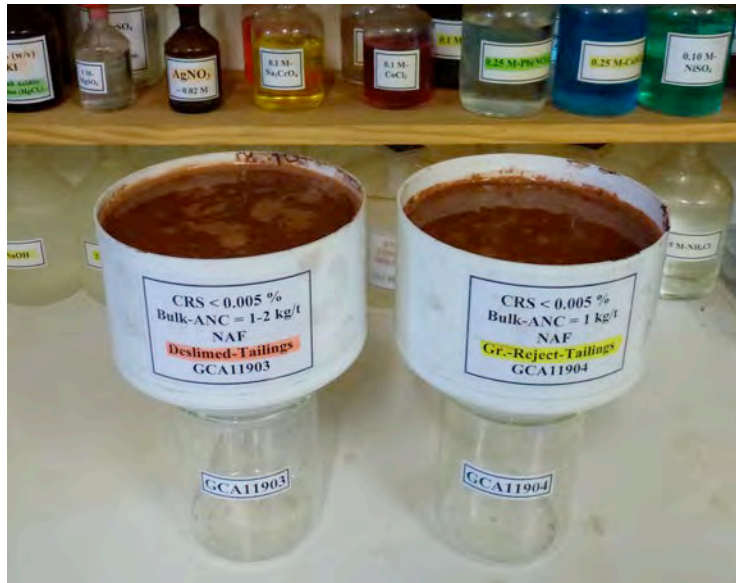
PLATE 7: Initial flushing (= "Cycle-0") of humidity-cells containing dry tailings-solids passed through 4.75 mm stainless-steel sieve prior to packing cells (columns) with 1.00 kg dry-solids of tailings. High-purity-deionised-water (HPDW) used for flushing.
