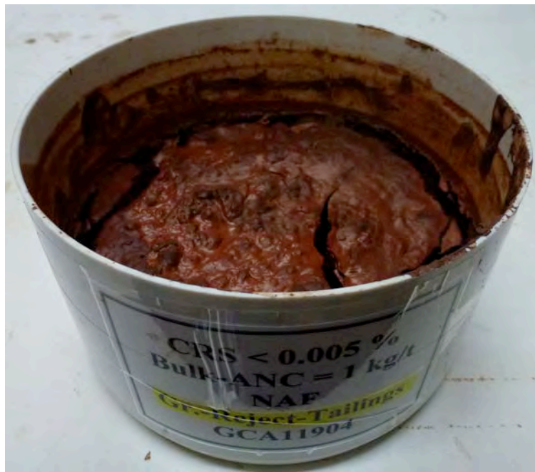
PLATE 8: Desiccation/shrinkage-crack formation during dewatering of Gravity-Reject-Tailings at 30 oC in incubator.
