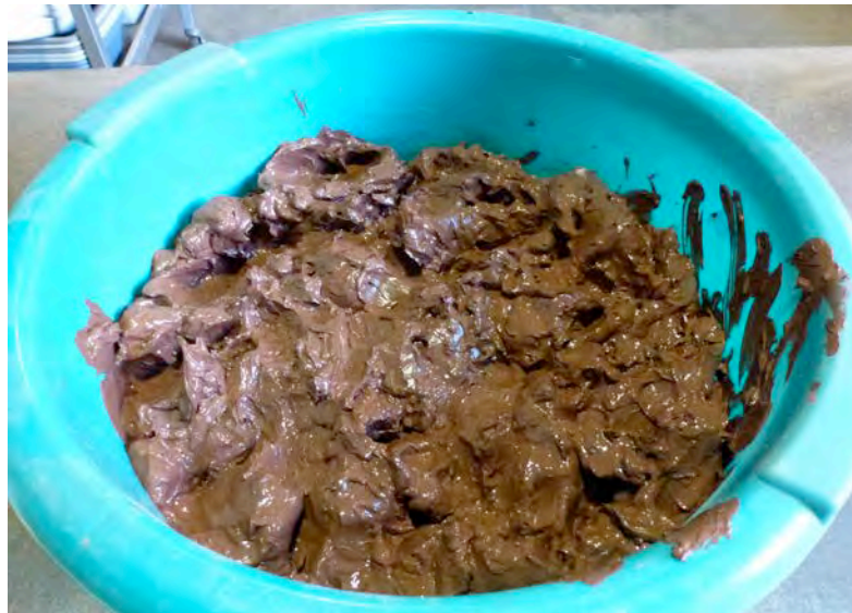
PLATE 3: Supplied 'wet' filter-cake of Deslimed-Tailings-Solids initially separated from plastic-bag (top photograph), and after homogenising via hand-mixing in a plastic bowl (bottom photograph).
